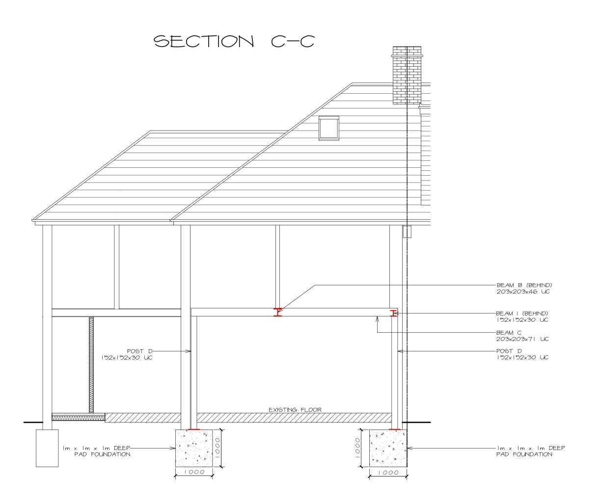
FOUNDATIONS TO BE 600mm WIDE, TRENCH FILL TYPE IN 1:2:4 CONCRETE. MINIMUM DEPTH OF IM BUT TO BE DEEPENED AS NECESSARY TO SUIT GROUND CONDITIONS \$ IN THE CASE OF ADJACENT DRAINS TAKEN BELOW THE INVERT LEVEL, FINAL DEPTH TO BE AGREED BY BUILDING INSPECTOR.
